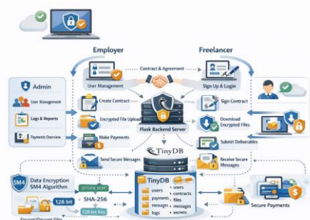
Fig. 1: Proposed system architecture of secure freelancer contract creation platform.
