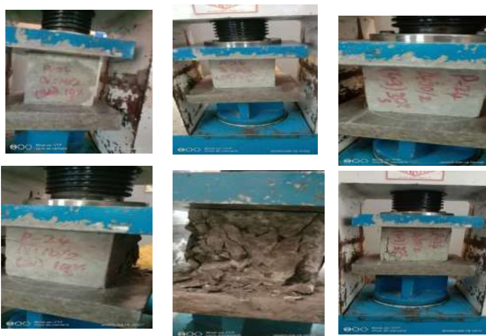
Figure 3: Before & after crack for replacement of FA by steelslag
