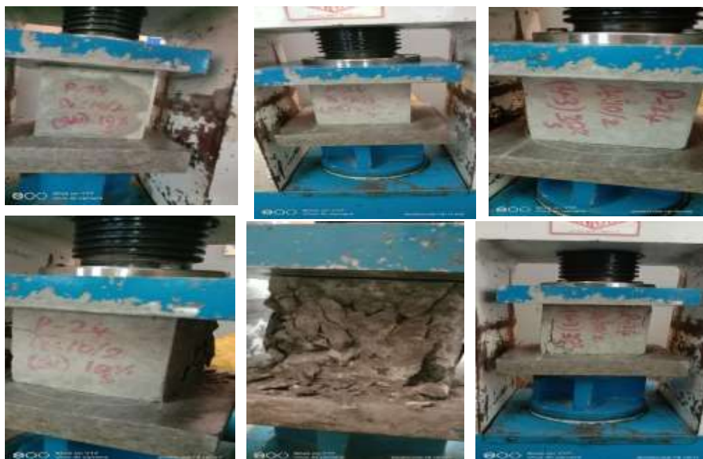
Figure 5: Before & after crack for replacement of FA by steel slag
