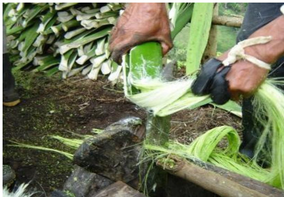
Fig 6.2: extracting the fiber from Sisal fiber plant
