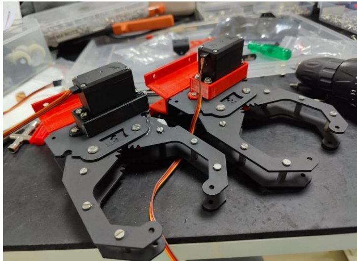
Fig. 6: Dual Servo Motor Gripper Mechanism for Robotic Manipulation
