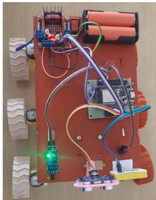
Figure 4: Top View of Rocker-Bogie robot showing electronic components integration
