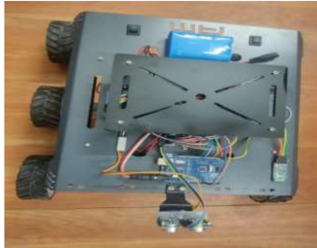
Figure. 3: Hardware prototype of gesture-based embedded system
