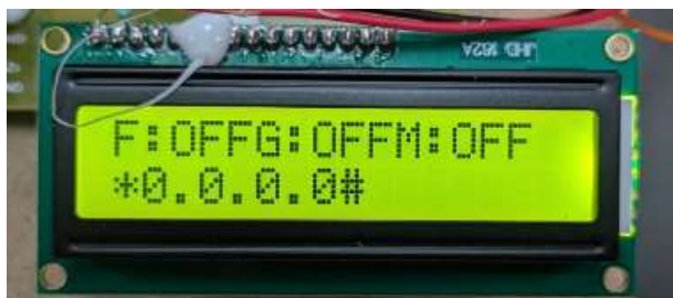
Fig 3. Real-Time Sensor Status Display on LCD in IoT Spy Robot
