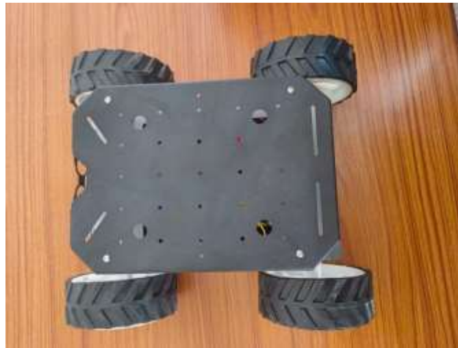
Fig. 3: Top View of Four-Wheeled Robot Chassis Showing Mounting Plate and Wheel Configuration
