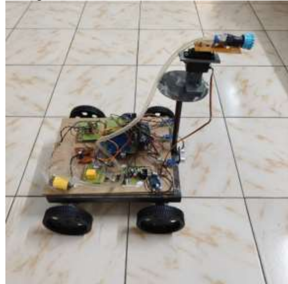
Fig. 4. Fully Assembled Fire Fighting Robot with Servo-Controlled Water Extinguisher Mechanism
