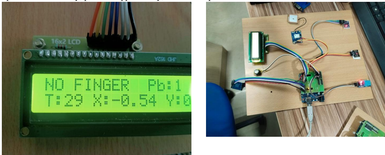
Fig. 2. Experimental setup and LCD output of the ESP32-Based biometric monitoring and tracking system
