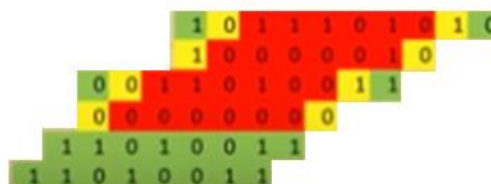
Fig 1.6: partial product addition, step1
